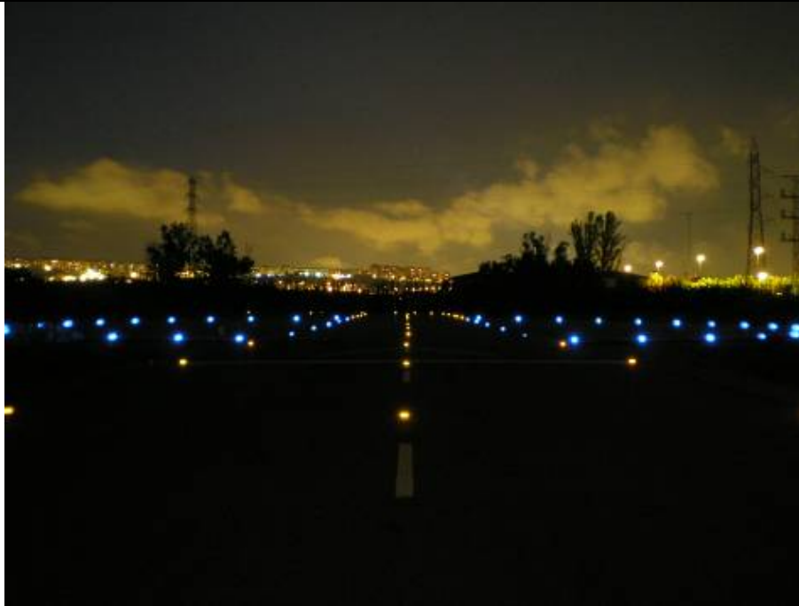
Image: Solar beacons illuminating the sound power track for night time testing.
