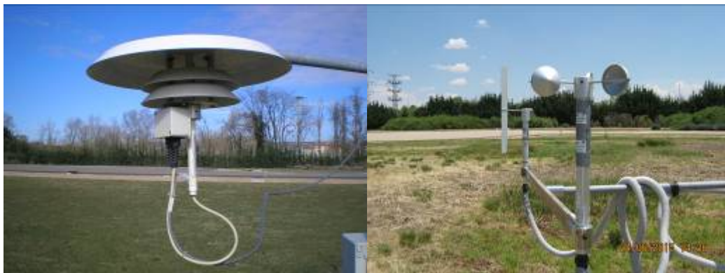
Image: CMA Weather Station. (Left: temperature sensors, relative humidity and pressure. Right: Wind direction and wind speed sensors).
