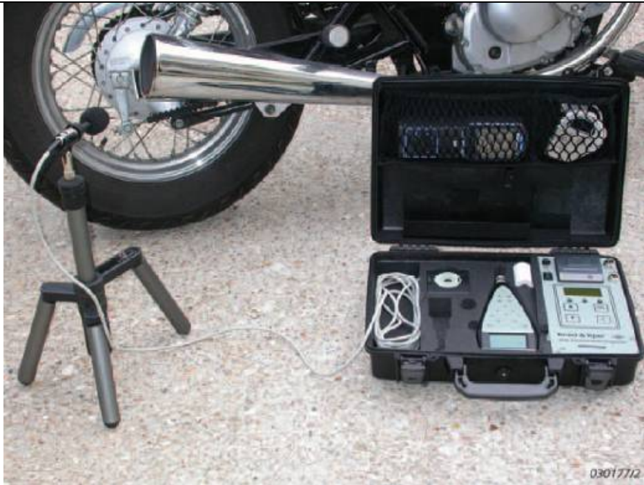
Image: Noise measurement of a stationary motorcycle in accordance with Directive 97/24/CE using Exhaust Noise Inspector Type 3638 (Brüel & Kjaer). Source: Brüel & Kjaer.
