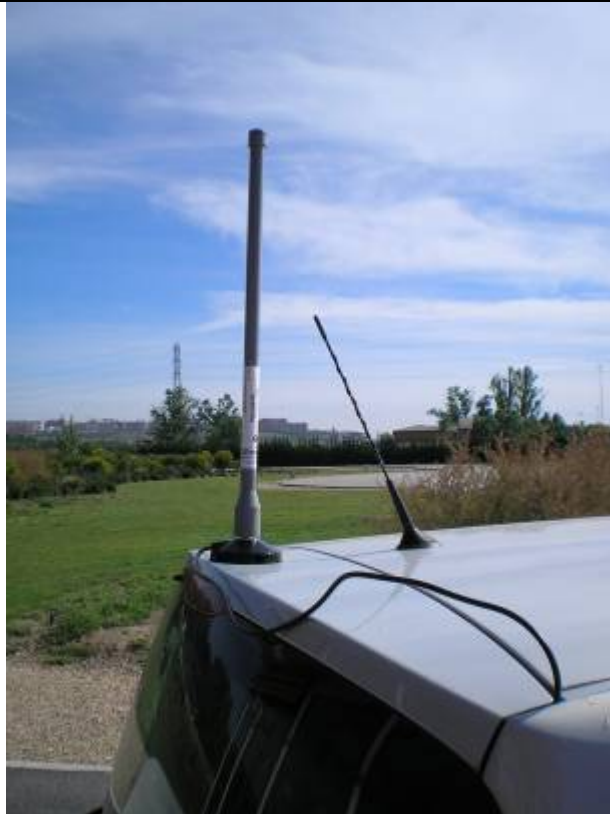
Image: Wi-fi antenna on the vehicle roof allows communication with the Pass-by control room.
