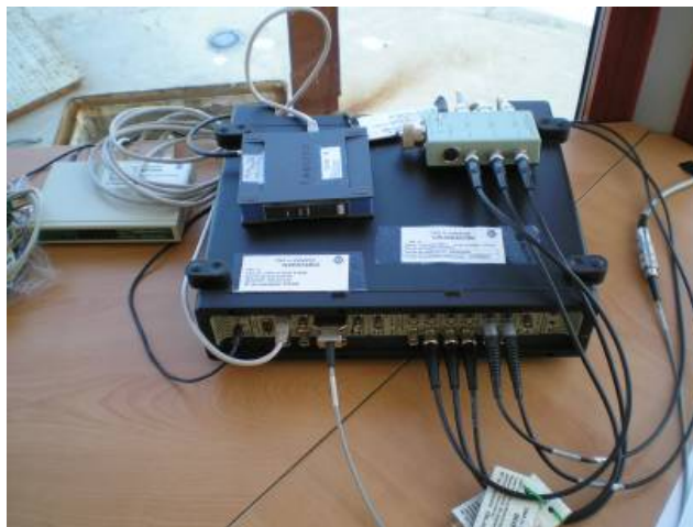
Image: Frontend data analyzer in the Pass-by control room, Brüel & Kjaer 3560C.
