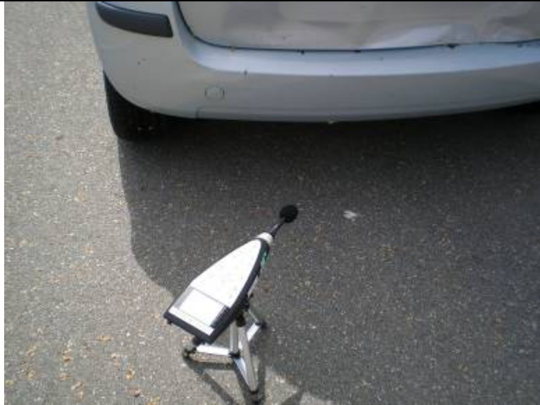
Image: Noise measurement of stationary vehicle using the Brüel & Kjaer Investigator sound level meter.
