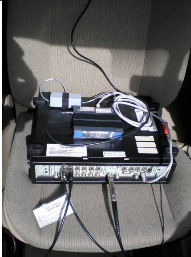
Image: Frontend for acquiring data from vehicle, Brüel & Kjær model 3560 C and wireless access point.
