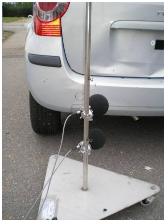
Image: Noise measurement of stationary vehicle using 4190L001 Brüel & Kjaer microphones and equivalent Pulse system, with one microphone measuring SPL and the other the determination of vehicle RPM through exhaust noise with Pulse Autotracker.
