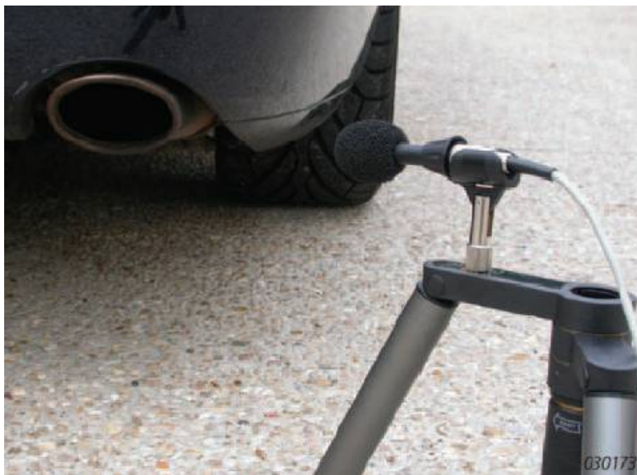
Image: Measurement of external vehicle noise using Exhaust Noise Inspector in accordance with Directive 70/157/CEE.
